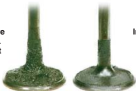
Intake Valve before P.i. Treatment
