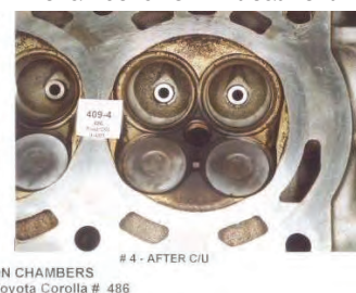
Picture H - Combustion chamber after P.i. treatment
