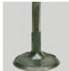
Picture E - Intake valve after P.i. treatment
